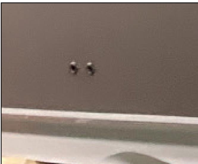
Bilge pump and air conditioner drain outlets
