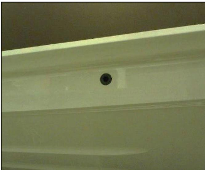
Starboard cockpit drain outlet
