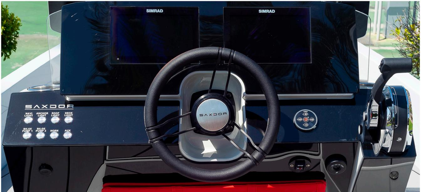
The electrical dials for the standard instruments are located on the port side of the steering console. These include lights, bilge pumps and the signal horn. For the operation of the navigation screens, please refer to the manual supplied by their manufacturer.
